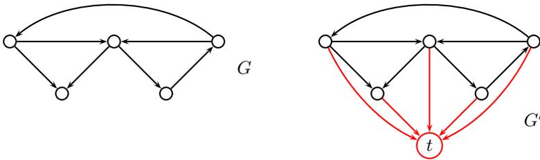
$G' = (V', E')$   $V' = V \cup \{t\}$ ,  $E' = E \cup \{(v, t) : v \in V\}$ ,  $\text{costo}(v, t) = 0, \forall v \in V$ .
